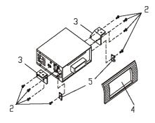
**Note:** The mounting box, outer trim ring, and the half-sleeve are not used for this method of installation.
